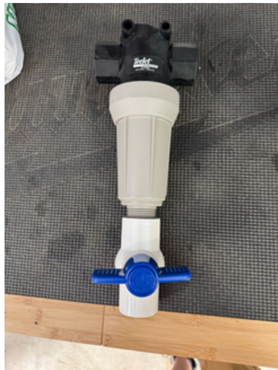
A 50-mesh inline filter assembly with a 1/4 turn ball valve for quick flushes.
