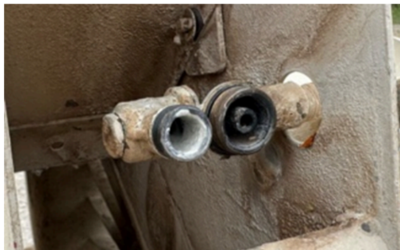
A clogged slotted strainer inside the nozzle body. Note that the inners of the check valve seem clear (a good thing).
