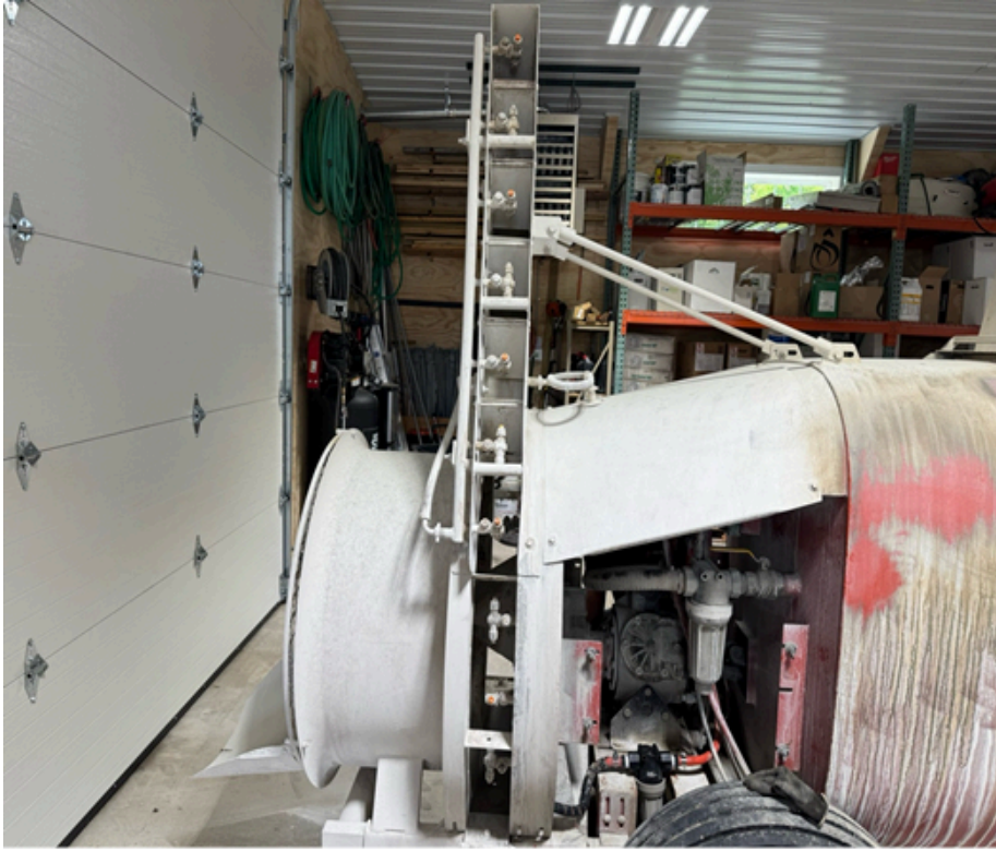
The new loadout. 02's in every second position, with no tip strainers, and a new inline filter on each side of the sprayer.
