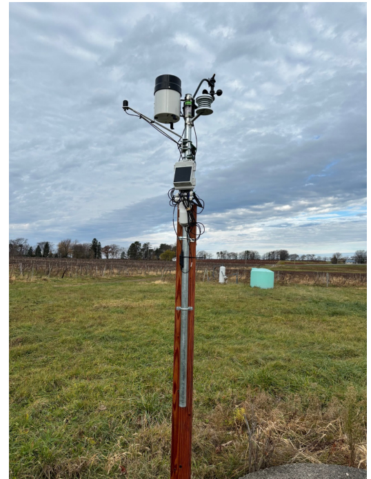
Figure 1 new Onset HOBO station set up Dunkirk (Route 5)
