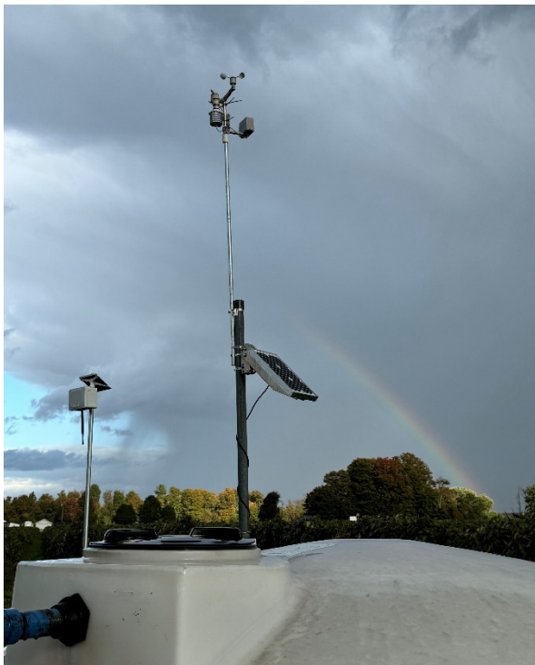
2. Photo of one of grape.ag's weather stations and gateways installed near a Concord vineyard.
