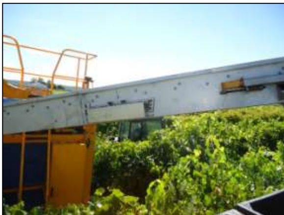
Image 1 Top Left: The weigh-frame embedded into a hole cut into the discharge conveyor belt tray. The front lip is set slightly higher than the tray so that the conveyor belt rests on the weigh-frame lip.
