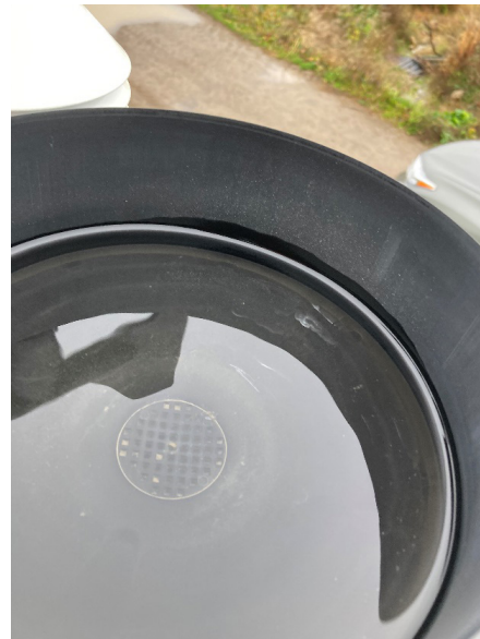
Figure 1 Standing water in rain bucket
