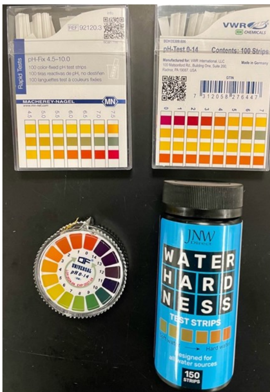
Photo 1. Examples of different pH strips and hardness strips. pH ranges from 0-14 and 4.5-10, hardness range 0-425 ppm. Price is about $10 for 100-150 strips.
