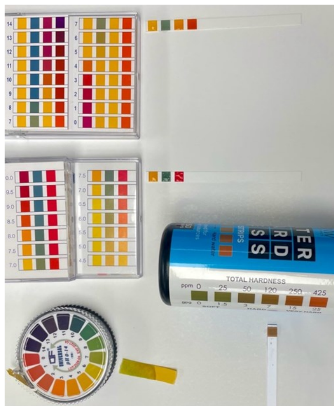
Photo 2. Easy, inexpensive testing of water pH and hardness using strips. Example of readings from sink water at Cornell AgriTech. The pH is between 7 and 7.5 with multicolor strips and between 6 and 7 with paper roll. Multicolored pH strips are more accurate than pH rolls. Water hardness is 7 gpg (120 ppm). Conclusion: this water needs to be treated by buffering and conditioning adjuvants.
