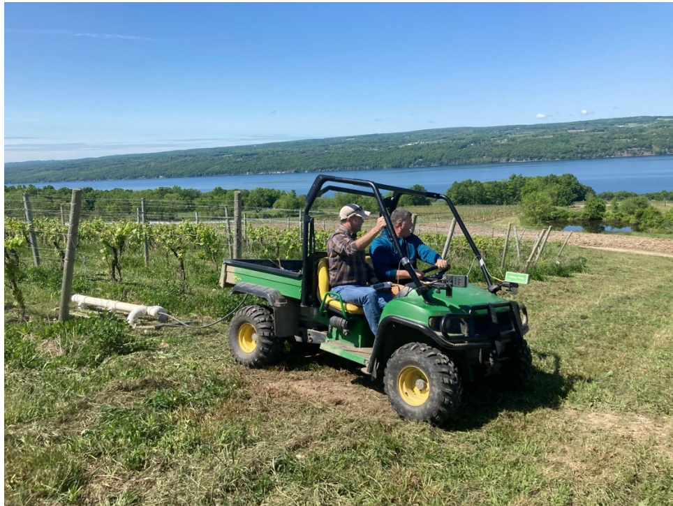
Hans and Terry Bates scanning a vineyard on Seneca Lake. The small boxes on the front are NDVI sensors that quantify the presence of green tissue. The sled being pulled behind is measuring the electrical conductivity of the soil at two different depths, which gives an estimation of several soils properties such as clay content.
