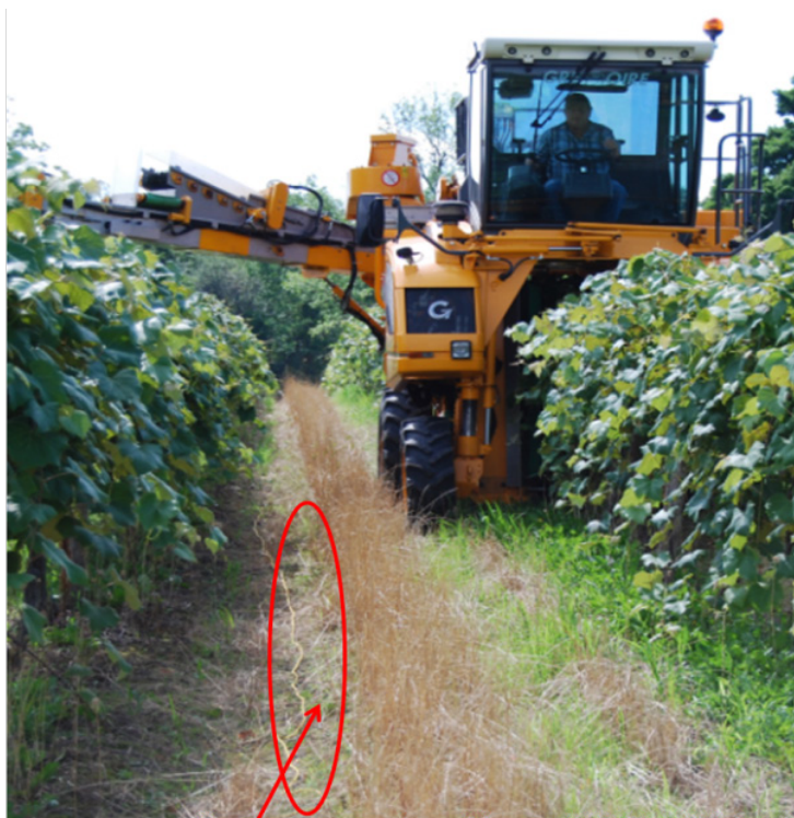
Length of rope used to guide harvester on distance of sample (determined by row width).
