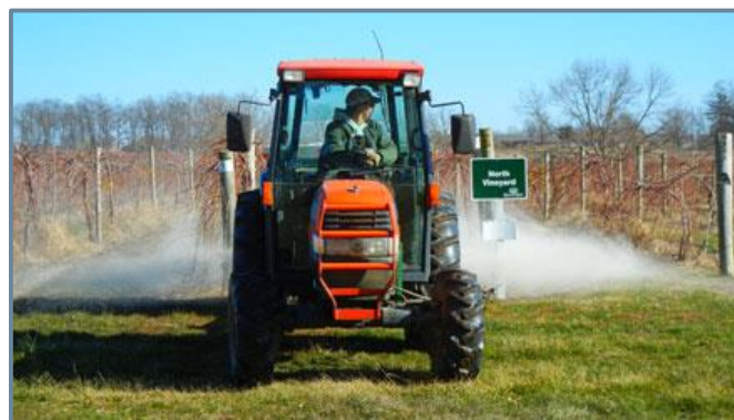
Figure 1 Lime application with Stolzhus lime spreader. Taken from Liming the vineyards . 2012. Missouri State University
