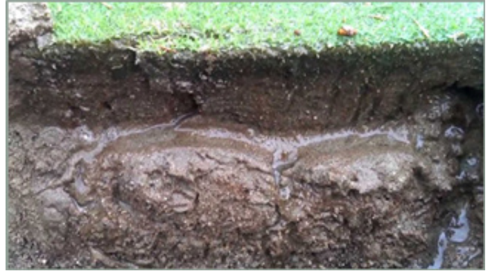
Figure 2. Soil Compaction Layer Illustrating Water Runoff. Photo by Jason Haines.
