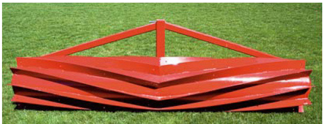
Picture 3: Crimper roller is an inexpensive tool that quickly terminates cover crop. Flexibility of timing has been a real issue for perennial crops.
