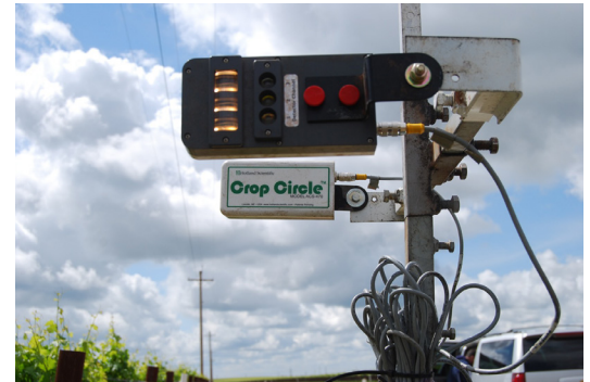
Measuring canopy with a crop circle sensor. Sensor is used to map relative vine size and other canopy attributes depending on the timing of the scan.
