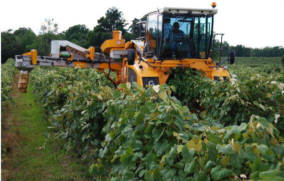
Thinning with variable rate shakers on Gregoire Harvester at Betts Vineyards
