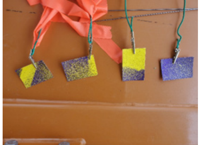
Spray coverage demo with water sensitive paper
