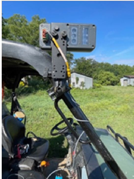
One of the NDVI sensors being used to improve crop estimation in Concord vineyards
