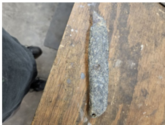
Debris removed from a spray tank during calibration
