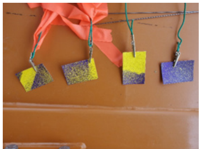
Spray coverage demo with water sensitive paper
