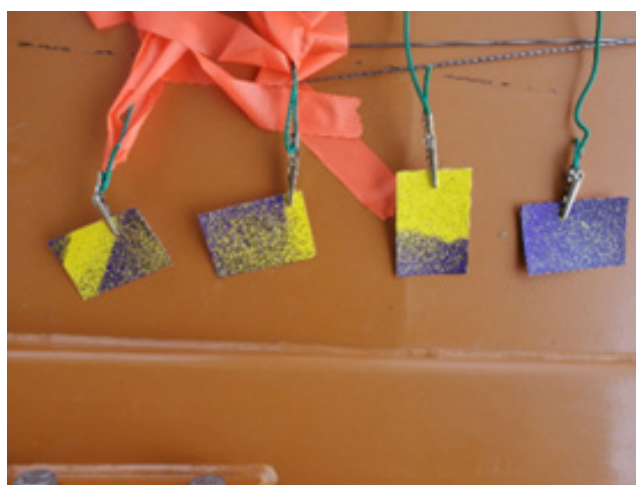
Spray coverage demo with water sensitive paper
