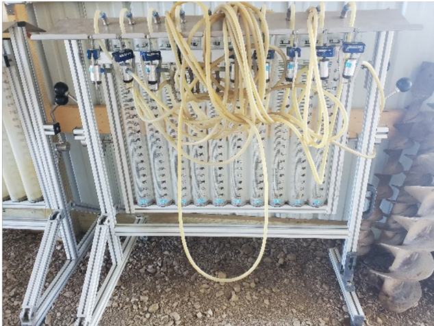
Customized equipment for pesticide sprayer calibration
