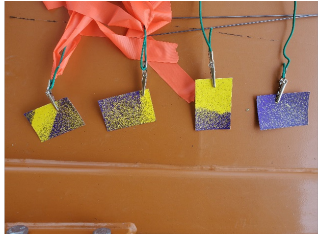
Spray coverage demo with water sensitive paper
