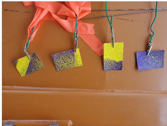
Spray coverage demo with water sensitive paper
