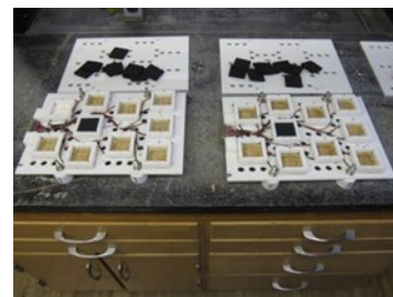
These trays can detect tiny heat spikes when ice forms inside a bud, which tells us the temperature at which it was killed.
