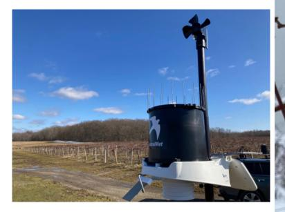
connection issues, the wind sensor was faulty and needs to be replaced. It has been initially set up without that sensor and has been reconnected to NEWA.
