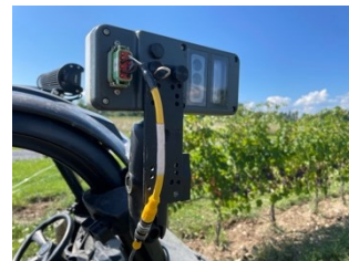
One of the NDVI sensors used to map vineyard variability during the growing season.
