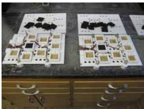
Trays used to hold individual buds during testing for bud cold hardiness at the Geneva Experiment Station.
